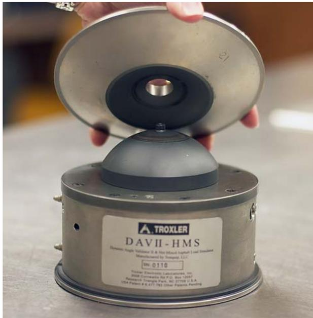
**Figure 4.7. Hot Mix Simulator (HMS) with Dynamic Angle Validation (DAV)**
