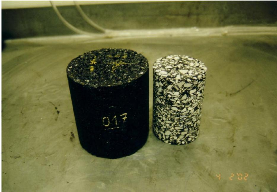
**Figure 4.2. Gyratory-Compacted and Cored Specimens**
